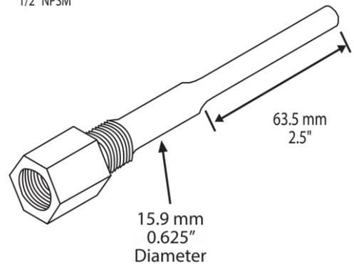
150 mm and up machined thermowells have a two step stem as shown. Welded construction have a 0.375" (9.5 mm) diameter.
